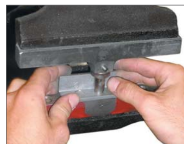
Bench vise used vertically as a press.
