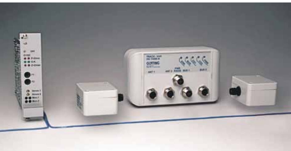
Track guidance using guide wire
