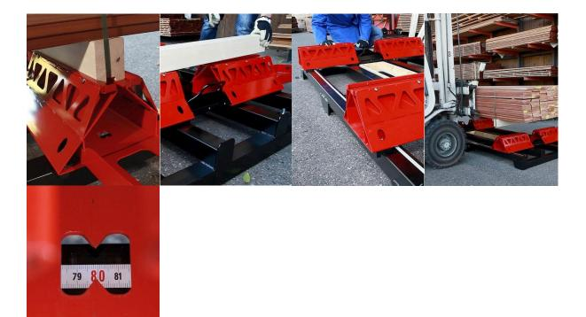
With the mobile sledge tunnel station scantlings can be embedded flexibly and exactly when strapping.
