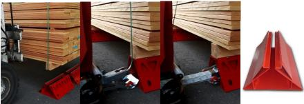
With the stationary sledge tunnel scantlings can be embedded when strapping pallets. The stationary sledge tunnels are fixed at the floor and can be used with any standard ErgoPack strapping system.
