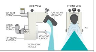
The AccuMist™ system combines Sono-Tek's unique Microspray ultrasonic atomizing nozzle with low pressure air to produce a soft, highly focused beam of small spray drops.
