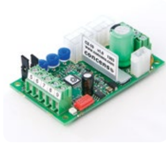
C2-10-PCB-00-0000-00 (board alone) 73 x 43 x 25 mm (L x W x H)
