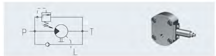
KM 1 pressure relief valve
