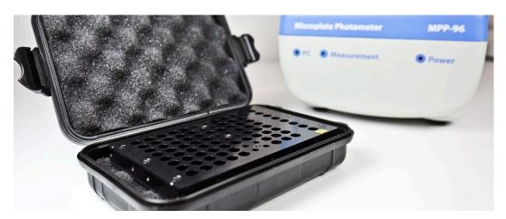
OD Plate is the quality verification instrument for microplate photometer MPP-96 HiPo. The instrument is designed to verify the accuracy and precision of measurements of the photometer at 6 levels of optical density: 0.3; 0.6; 1.0; 2.0; 3.0; 4.0 OD. The instrument is supplied with the following verification wavelengths: 405, 450, 492, 540, 570, 620 and 650 nm. Additional verification wavelengths are available in the range from 400 to 700 nm.
