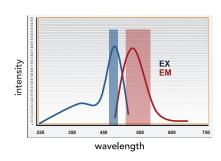
Variable bandwidth selection from 3 nm to 50 nm in 1 nm increments offers great versatility and is ideal for fluorophores with small Stokes shifts, broad excitation/emission bands, or for FRET and multiplexed assays where wavelength specificity is critical. Four holographic gratings are used to eliminate stray light and increase signal-to-background ratios, ensuring consistent performance for every read.
