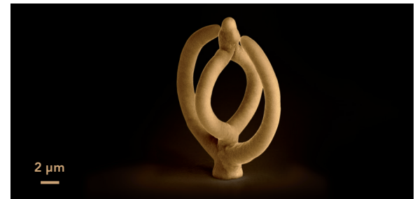
PRINTED OBJECT. Printed in one single step and without support structures.
