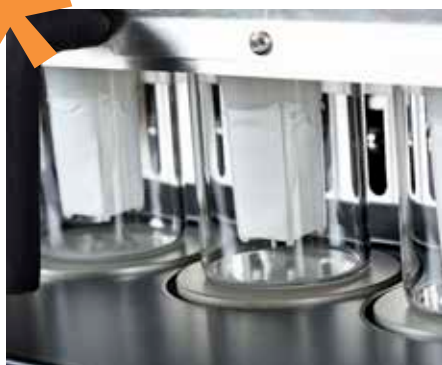
The unique, patented Hydrocap filter contains the sample all the way from initial weighing through hydrolysis to final extraction.
