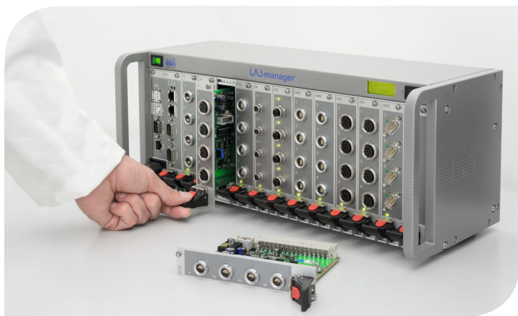
Easy „on-the-fly“ change of the slide-in modules
