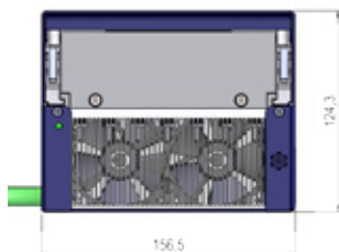
Front view & dimensions of all ODT ® versions
