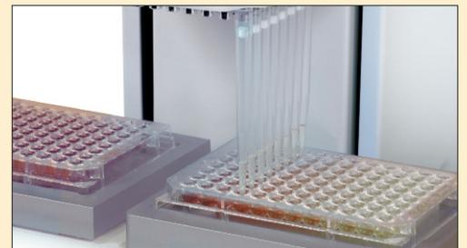
Performing serial dilutions and mixing of entire plates is easily accomplished. The number of mixing cycles and mixing speed can be exactly defined.
