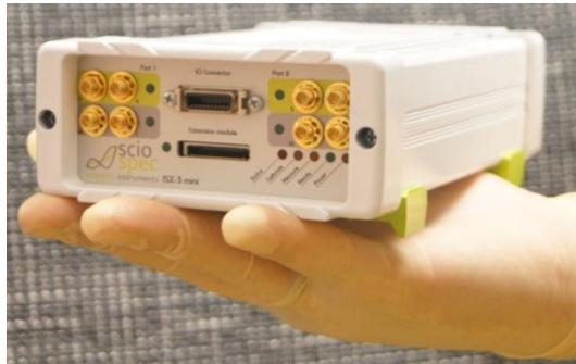
Sciospec ISX-3mini – Electrical Impedance Spectroscopy
