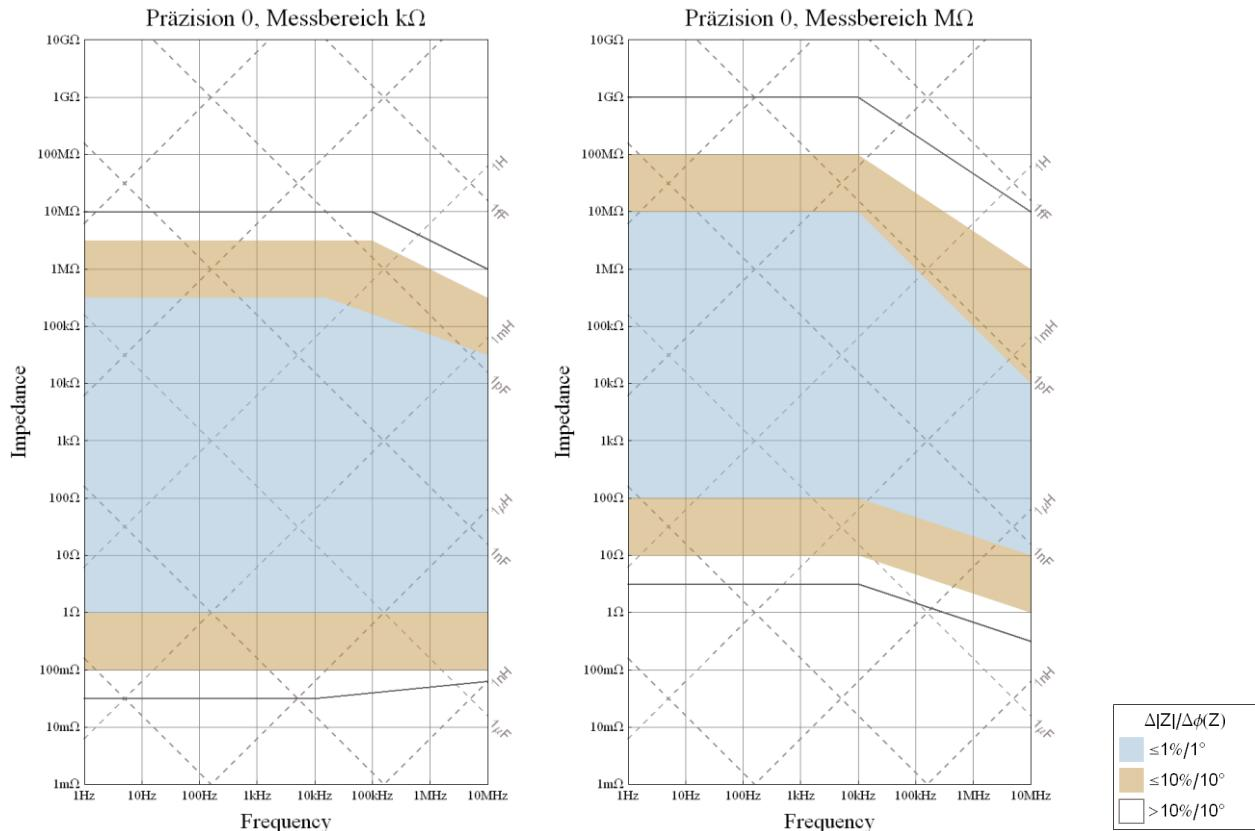
All specifications refer to measurements done with a Sciospec ISX-5 in combination with the Sciospec MEArack. The signal amplitude is set to 100mV and the frequency range to „<10MHz“. Measurements done, using the BNC connectors show very similar results.
