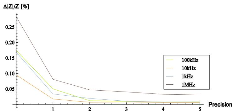
The diagram on the left shows the influence of the precision settings on the accuracy and time for the measurement of an impedance value at the specified frequency.
