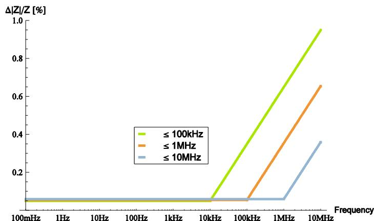
The choice of the frequency range also affects the accuracy of the impedance measurement. This relation is shown schematically for one measurement.
