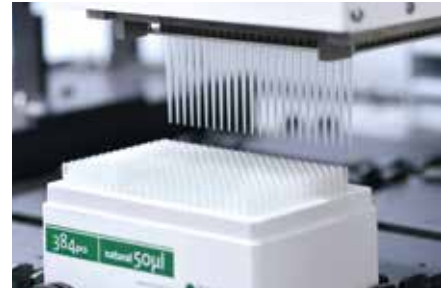
Multiple Channel Arm 384 picking up one column of 50µl tips
