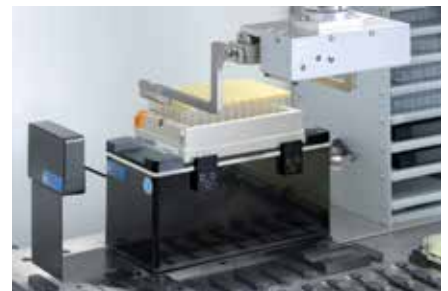
Robotic Gripper Arm with eccentric grippers loading a 2-D bar code reader
