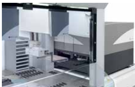
Side integration of Tecan Spark 10M multimode reader
