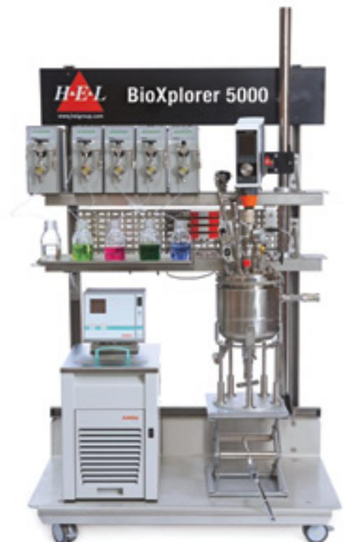
2 L Bioreactor rated to 10 bar with SIP, with custom configurations
