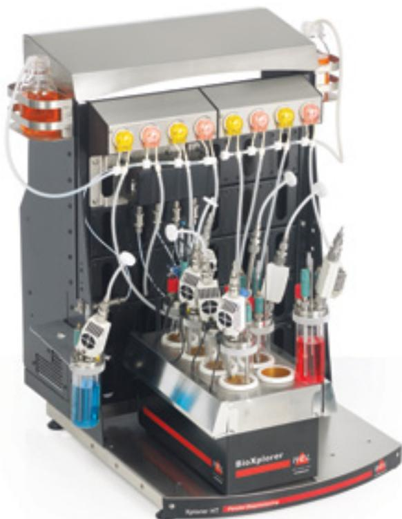
8 parallel reactors totally independent in temperature, stirring and all other process conditions. Multiple blocks can be combined
