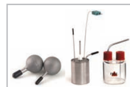
Range of test cells for PHI-TEC and TS U
