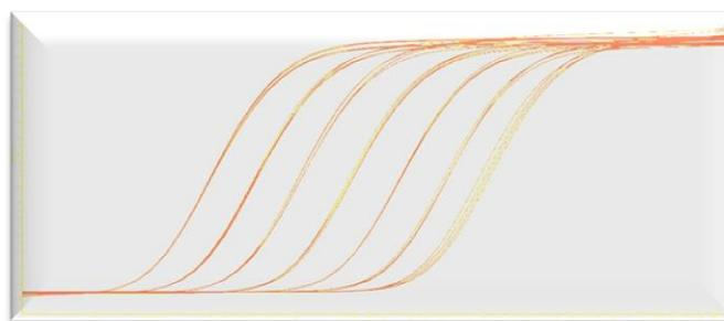
*4 pg, 40 pg, 400 pg, 4 ng, 40 ng, 400 ng and 4 µg of mouse total RNA were used for cDNA synthesis under the standard qScriber™ cDNA Synthesis Kit protocol conditions. An aliquot from each reaction was taken for subsequent qPCR with ORA™ qPCR Green Mix to amplify a 70 bp fragment of the mouse RN18S gene. All reactions independently from the initial amount of RNA were 100% efficient.*
