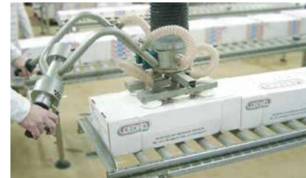
Adjustable operating handle in V2A steel design
