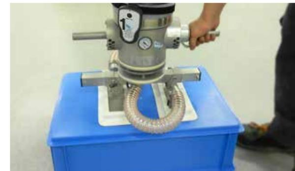
Operating knob in V2A steel design with wireless transmitter
