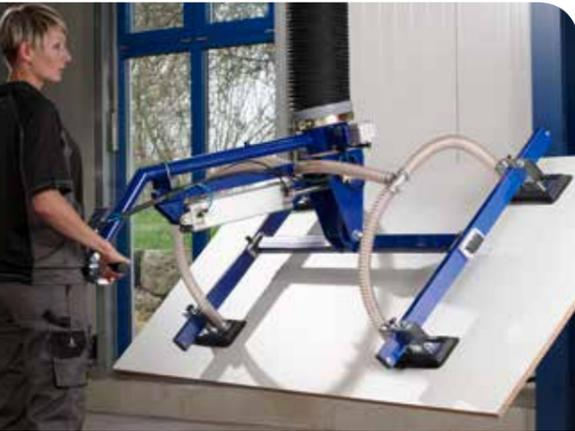
MAXI-LIFT with swivelling unit for plates up to 300 kg
