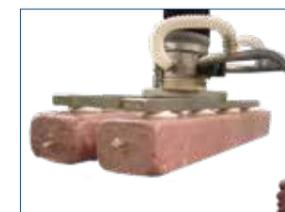
Suction cup system for food (in V2A steel design)
