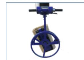
Suction cup for handling chimney flue tiles
