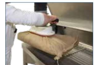
Sack lift (in V2A steel design)
