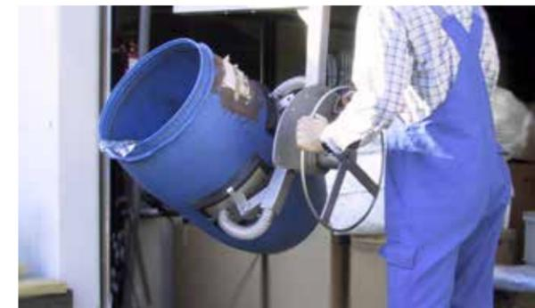
Manual slewing by handwheel
