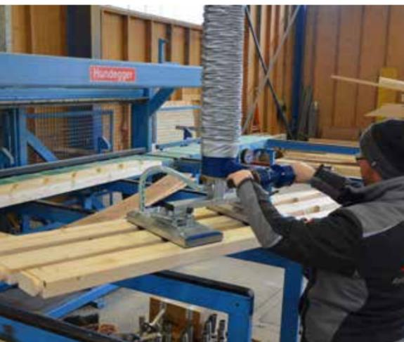
MULTI-LIFT vacuum gripper suction cup for wooden strips
