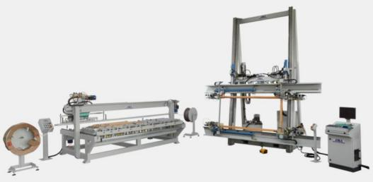
When supplied together with a TITANPRESS clamp, it allows gasket insertion while assembling the previous frame, significantly increasing productivity.
