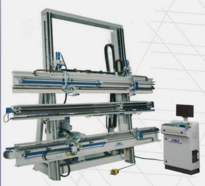
It is equipped with an electronically controlled, automatic variable-pitch rack which allows the operator to quickly and precisely position louvers, with no need for manual adjustments when size or typology of the louvered shutter change.
