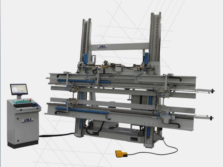
Pressing movements operated by 4 independent CNC controlled axes
