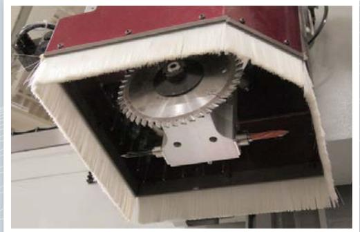
Multi-drill blocks are available with an optional X+Y Grooving Saw.
