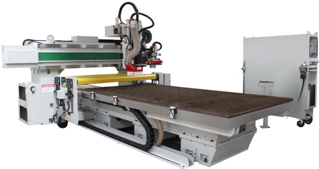
The optional roller holddown system is designed to apply vertical (downward) pressure to aid the vacuum system in securing parts in a nested-based application that cannot be held properly via vacuum alone or for multiple sheet stacking.
