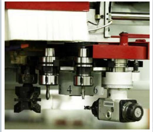
All Anderson CNC Routers include Aggregate Capability as standard and include an aggregate ready tool changer.
