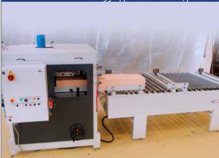
Splitter (H 100 - 250 mm) / Splitter (up to 100 and up to 250 mm thickness)
