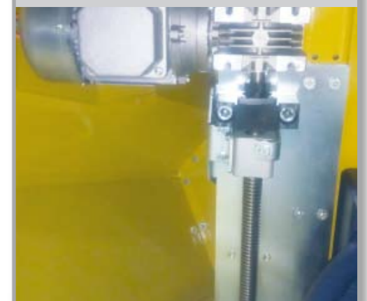
Electrical saw blade height adjustment (option)
