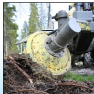
The T21.b is available with hydraulically-powered discs or rotating discs.
