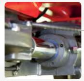
**Designed for heavy loading** due to its solid steering axle and centrepiece construction.
