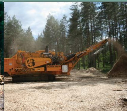
Chip logs into various size chips at rates up to 200 tons per hour!
