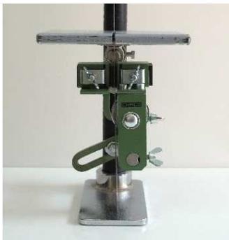
The model M30 is also available in the **M30 Hu** version with a H-shaped lower blade guide. This can be mounted even closer to the table and thus provides an additional stability increase. W 140, H 150, D 70 mm.
