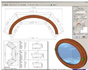
**POWERWIN** is the ideal CAD for the parametric design of solid wood doors, flush doors, shutters, standard and special doors and windows. **POWERWIN** is easy to use: the enduser is guided through all the designing phases, from the selection of shape up to the arch splitting into segments. With **POWERWIN** t is possible to configure all the parameters of the elements making up a window or a door: frame, openings, overlapped parts, sections,
