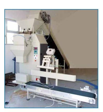
We can provide semiautomatic bagging machines with capacity up to 150 bags per hour, full of net weight scale, evacuation belt for the bags and welding thermal resistance. We also have layer palletizers used and reconditioned.
