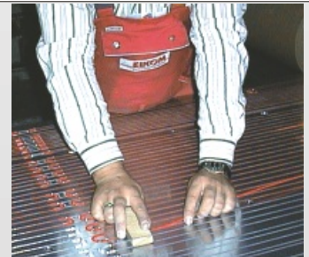
Quality up to the smallest Detail . The "bends" in the centre of the platen to compensate for thermal expansion can be seen. ( picture taken during production )
