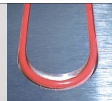
Quality up to the smallest Detail . The "bends" in the centre of the platen to compensate for thermal expansion can be seen. ( picture taken during production )
