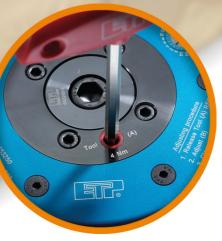
The extreme precise adjustment is easily done on the adjusting device by using the special designed bits. Each snap is equal to 0.01 mm movement between the two profile tools.
