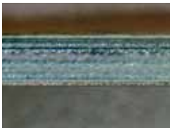
Cut edges of multi-layer film in detail
