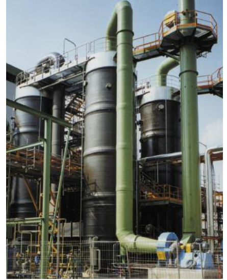
Two-Line double WESP in glass fibre (FRP); separation efficiency > 99.7 %
