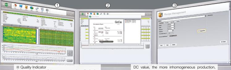
A clear indication of the current panel quality is the quality indicator. All measured values of a panel are compressed and represented as a quality key on a scale, similar to a speedometer.
