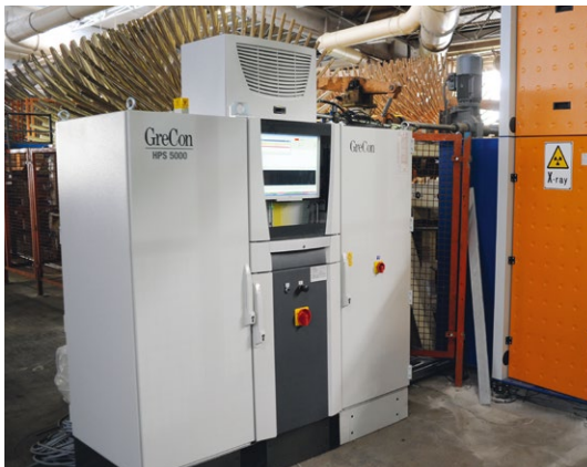
HPS control console with visualisation like in control station
