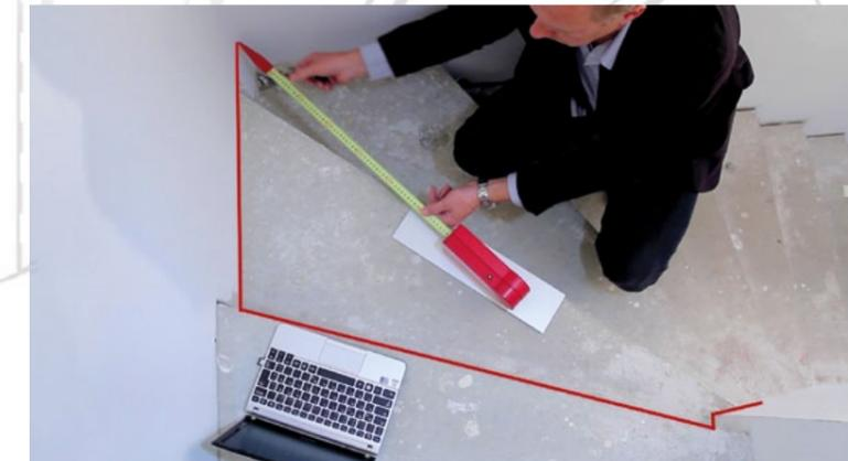
With the stairbox measuring unit, all coordinates from the measuring tip are detected with high accuracy and then transmitted via Bluetooth to the *Stairbox software* installed on the netbook. The measured step parameters are transmitted to the software in real time and then displayed on the screen which enables immediate visual control – missed or incorrect measurements and transposed numbers are a thing of the past!
