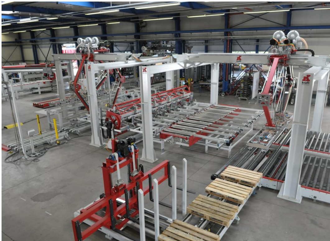
Portals for stocking of insulation boards
