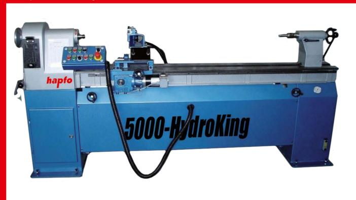
For the big-lot production and to satisfy highest demands on precision, the 5000-Hydro-King presents all technical advantages, which are charcteristic for an efficient hydraulic copying lathe. The 5000-Hydro-King is a very precise and powerfull machine in heavy grey cast iron and first-class workmanship made in Germany. The 5000-Hydro-King can be equipped with hydraulic scanning of the template or the original workpiece. The turning of thin part is also possible due to the follower-rest.
