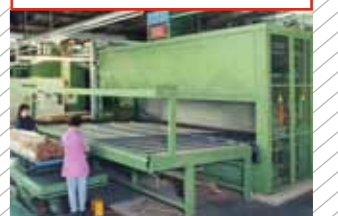
Press dryer outfeed system
