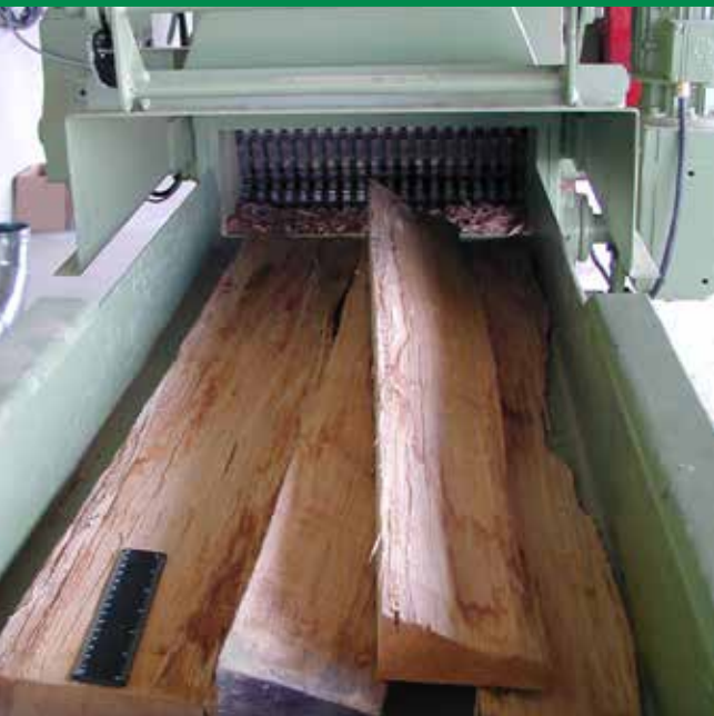
Feeding vibration conveyor / infeed rollers
