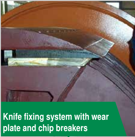
Chipping drum with special chip breakers
