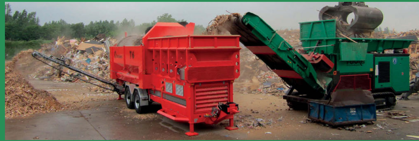
HAAS HDWV Primary Crusher with Drum Screen
