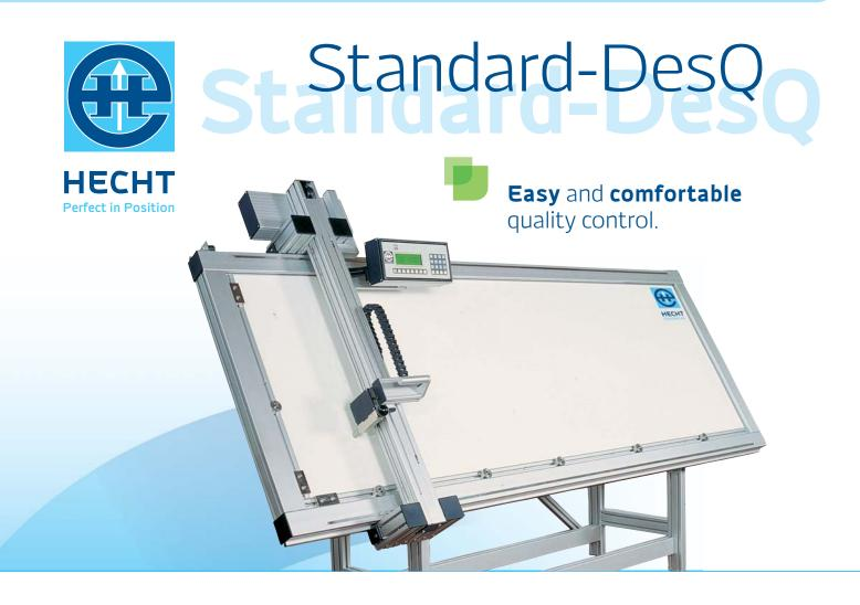
The measuring table Standard-DesQ is suitable for exact manual measurements of drilling holes and external dimensions. No software is needed for operation. The Standard-DesQ can also be delivered with Z-axis for depth measurement, vacuum suction system to fix parts and turred head for easy operation and fast measurement.
