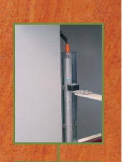
Linear position transducer The linear position transducer has two functions - it surveys the pressing area, ensuring that doubling-up does not occur and in addition, it stops all movement and generates a malfunction prompt when workpieces are not centered.
