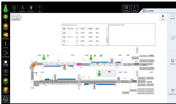
Fig. 2: woodFlex: Control and visualization of flexible production cells and their part flow
