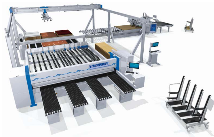
Fig. 3: HOMAG is placing a particular focus on woodworking shops once again in 2017. Here: A completely networked sawing-storage-nesting cell
