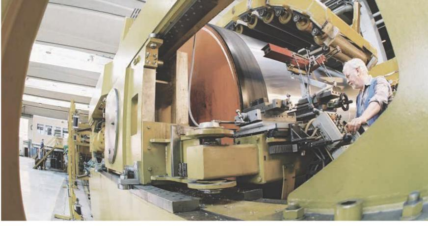
Specialised machinery and production techniques are used in the manufacture of steel belts for WBP double belt presses in order to meet the fine tolerances required by this industry
