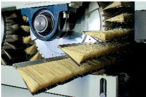
RotoMaster Equipped with Smart-Flex sanding strips. Quick and easy changing of strips by using split end caps.
