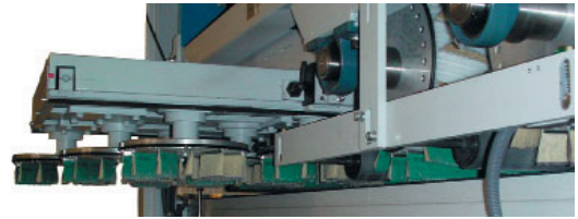
Simple changing of sanding strips by pulling out the disc station on both sides
