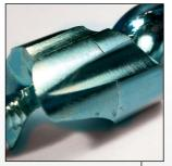
The sunken stepped drilling head achieves lower total friction during drilling through the partial focused warmth development. The ELITE bit is exposed to very low stress behind the stepped drilling head. This allows a very efficient chip flow, also in extremely deep drillings! Higher rotations than in common auger bits are recommended.
