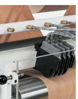
After the foil from the wide roll is slit by the pneumatic roller cutters it is wound into straight-edged narrow rolls. The length is indicated on a meter counter.
